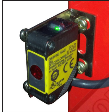
Power on & not aligned
